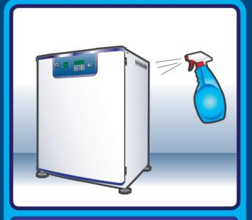
CO<sub>2</sub> Incubator needs to be cleaned with a disinfectant or detergent first and then rinsed with sterile water followed by 70% alcohol.
